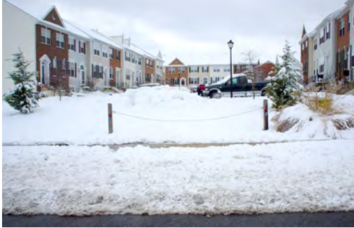
Figure 3.10. The same fire lane covered with snow. Access is blocked by a mound of snow plowed from the adjacent parking lot.
