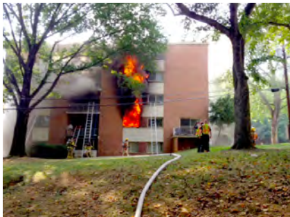
Figure 6.1. A building with poor apparatus access and challenging terrain for firefighters stretching hose lines and placing portable ladders.
