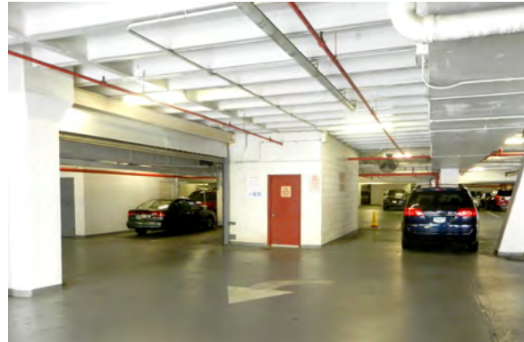
Figure 11.17. A fire command center (behind the red door) in a parking garage. To access this room, firefighters must make entry through a steel vehicle entry gate; however, it opens automatically upon fire alarm activation. A nearby car fire could render this room inaccessible even though its walls and door are fire-rated.
