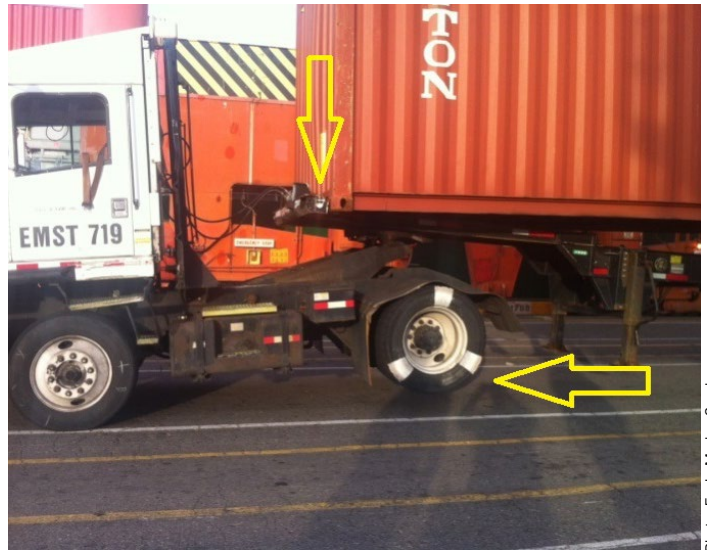
Container is partially disconnected causing the chassis to lift.
