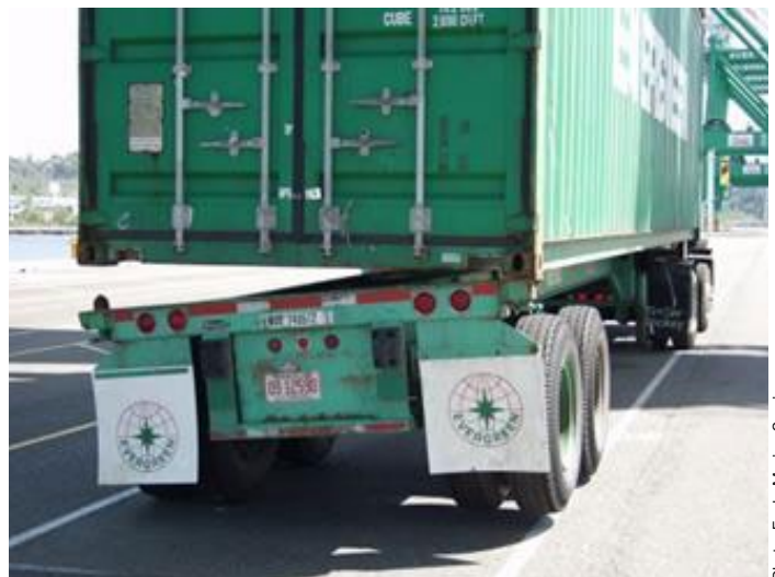
Semi-tractor with partially disengaged locking mechanism.
