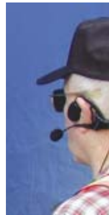
Detail of “temple-transducer” style radio headset.
