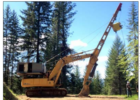
Figure 2: Excaliner with excavator pressed to the ground.
