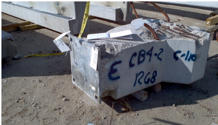
Fig. 53 – Column B4 upper segment above splice after demolition
