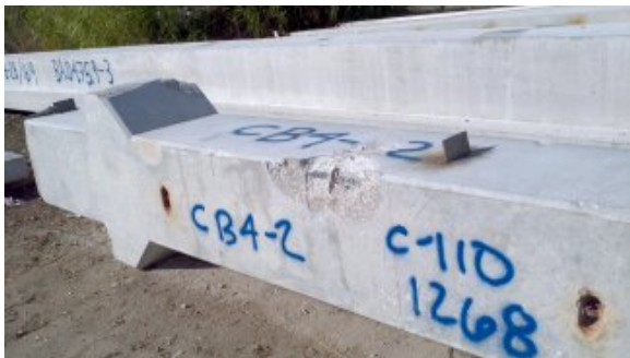
Fig. 53 – Column B4 upper segment above splice after demolition
