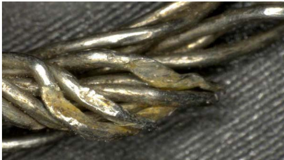
Figure 51 - Gouging and crushing damage on the wire ends at the point of failure
