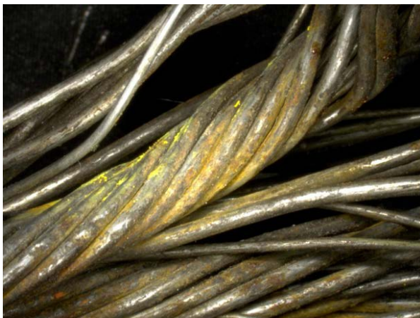
Figure 43 - Yellow paint-like substance on wire rope away from the fracture surface
