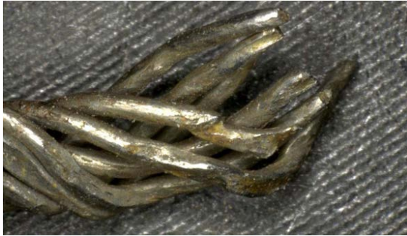
Figure 49 - Inner core wire ends showing evidence of scraping, gouging and abrasion
