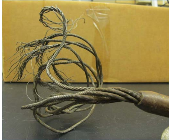
Figure 42 - Failed wire rope sling.
