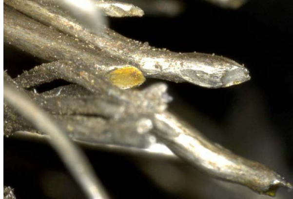
Figure 46 - Close-up of Yellow substance on fractured surface
