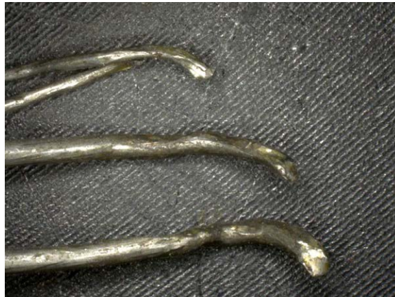
Figure 52- Hooked ends are indicative of being pulled around a sharp corner
