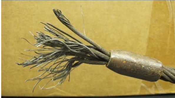
Figure 41 - Failure next to swage on the wire rope sling.
