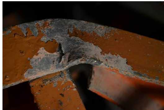
Figure 54 – Cuts and bruises from abrasion of wire rope
