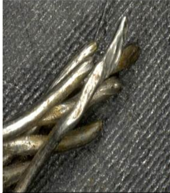
Figure 50 - Evidence of gouging, abrasion and crushing on the failed ends
