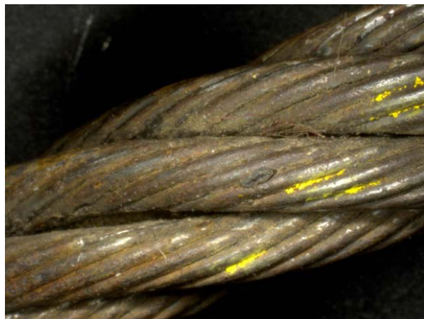
Figure 44 - Yellow paint-like substance laying in the valleys of the wire rope
