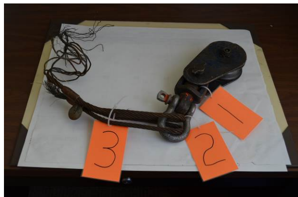
Figure 40 - Top block and broken sling
