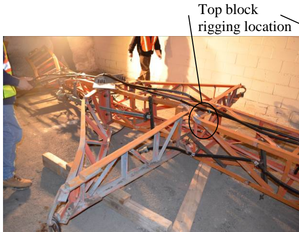
Figure 37 - Top block rigging location
