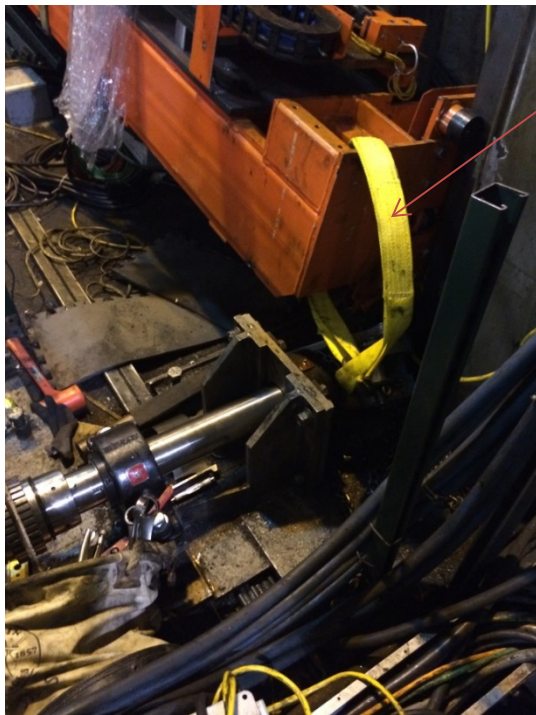
Fig. 5 – Attachment point for come-a-long
