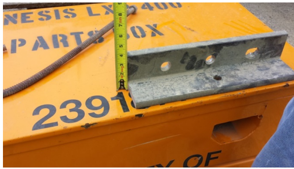
Figure 21 – 4x4x3/4" angle used at abutment #2
