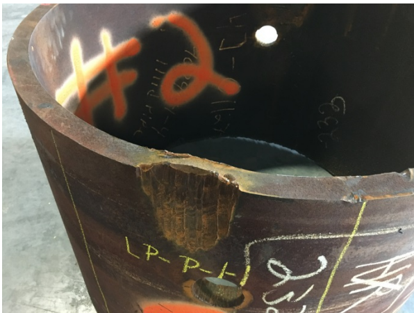
Fig. 36 – Deep indentation on the south side of pile #1
