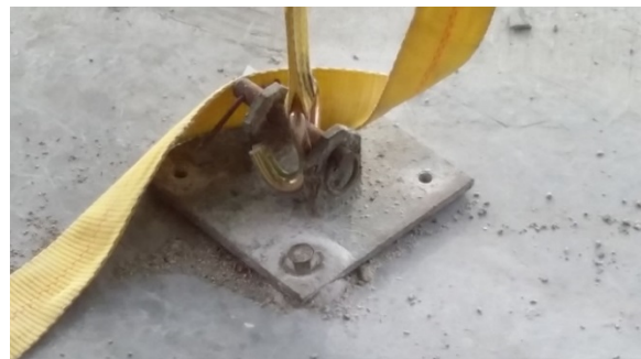
Fig. 25 – Ratchet Strap anchoring.
