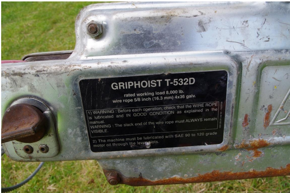
Figure 15. Lemay Come-a-long Used On-site
