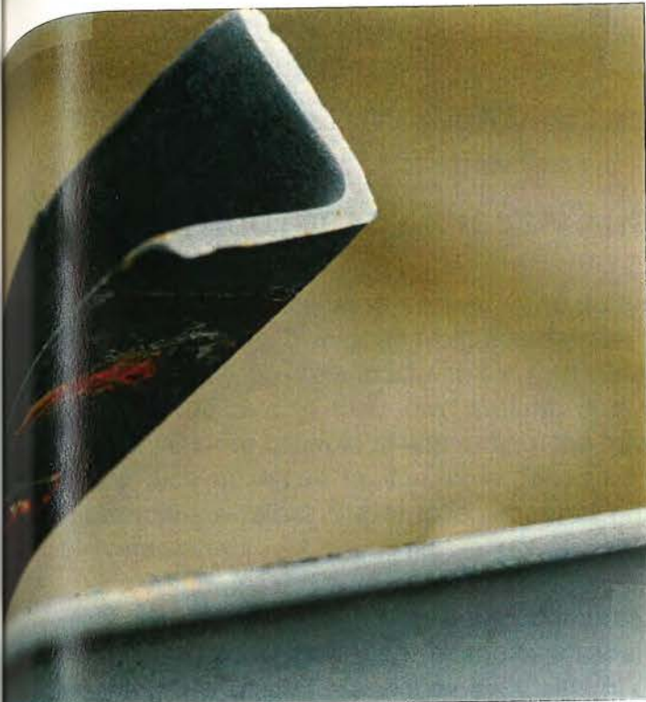
Fractured Welds in Diagonal Member Spacers Between Top and Bottom Chords
