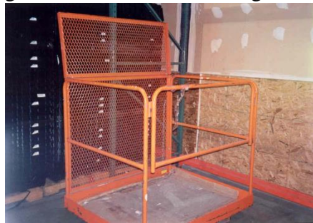
Photo: approved lifting platform with guardrails and metal mesh guard
